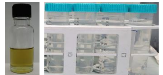
Crude and purified PMMA
